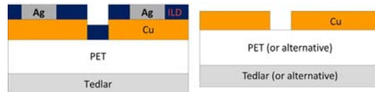
Figure 2: Cross section drawings of conductive back-sheet foil, left, first generation, with insulation lacquer (ILD) and plated Ag contacts, right, second generation, with no insulation lacquer and no Ag contacts
