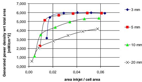
**Figure 4:** Cell size model calculation and area inkjet vs. cell area
