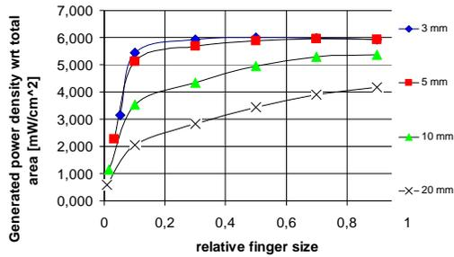
**Figure 3:** Cell size model calculation and relative finger length
