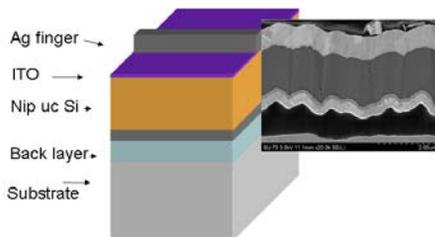
**Figure 1:** Si: nip cell structure with SEM picture and corresponding layer definitions
