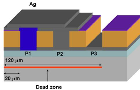
**Figure 2:** Si: nip cell interconnection structure with the dead zone (blue: isolating ink, gray: conductive Ag ink)
