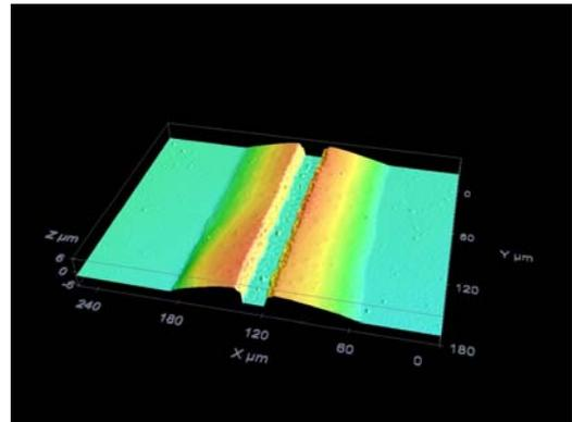
**Figure 8:** Laser ablation placed in 125  $\mu\text{m}$  wide inkjet line. Laser width 20  $\mu\text{m}$
