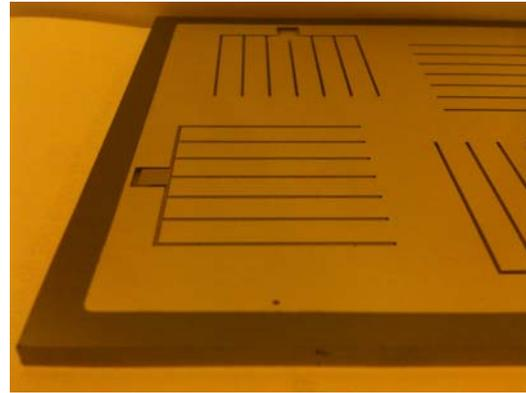
**Figure 7:** Inkjet printed Ag electrode structure inside laser ablated structure
