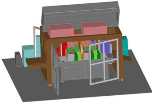
**Figure 9:** Produzo laser system inside laser safety cabinet
