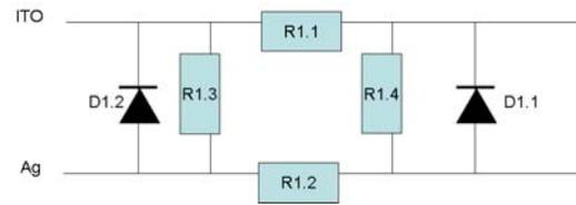
**Figure 5:** Steady state electrical model of the P1 scribe
