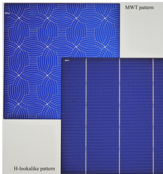
Figure 3: ECN's Circle MWT pattern (top left) and the H-lookalike MWT pattern (bottom right)
