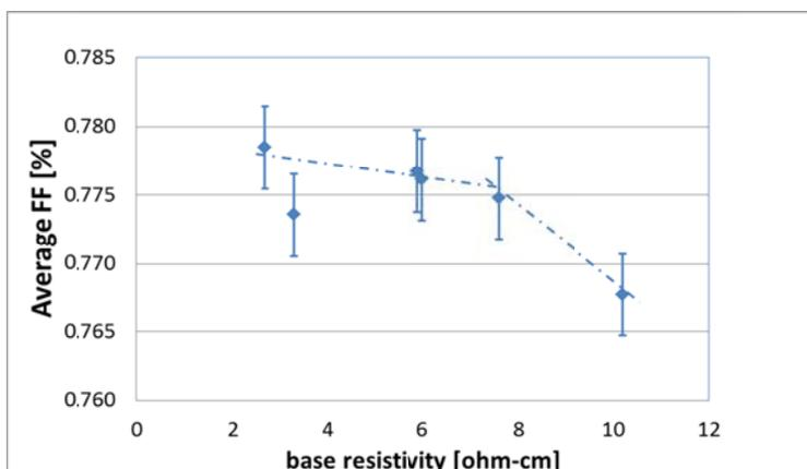
Figure 4: Average FF as function of the base resistivity of the n-Cz material.
