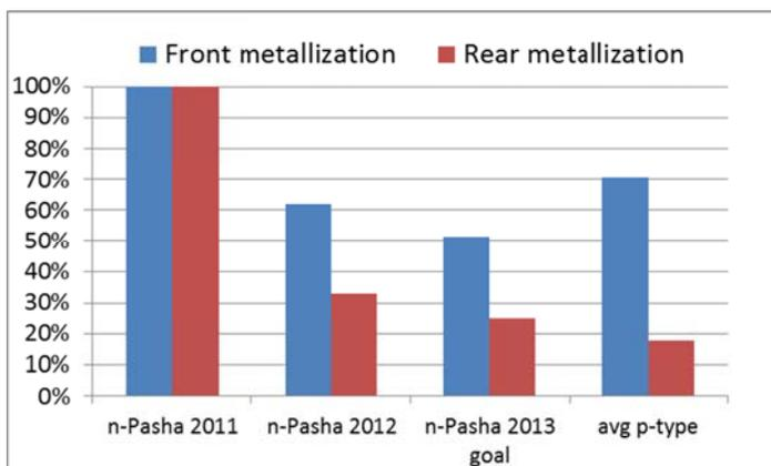
Figure 5: Relative silver reduction for front and rear metallization for n-Pasha, and comparison to average usage of silver on p-type cells
