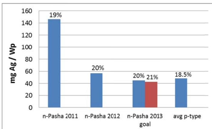
Figure 6: Silver consumption per cell per output power (watt-peak) for n-Pasha cells in 2011 (19% efficiency), n-Pasha cells in 2012 (20% efficiency) and n-Pasha cells with target Ag reduction for 2013 (shown for both 20% and 21% efficiency). All are compared to p-type cells with average 18.5% efficiency.
