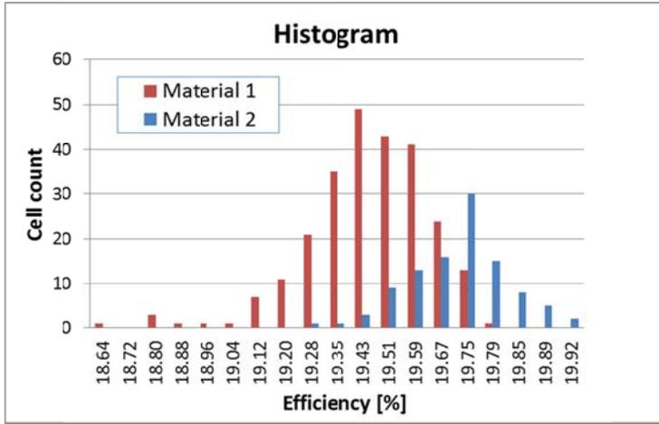
Figure 2: Efficiency distribution of >300 n-pasha cells fabricated on 2 different types of base n-Cz materials.
