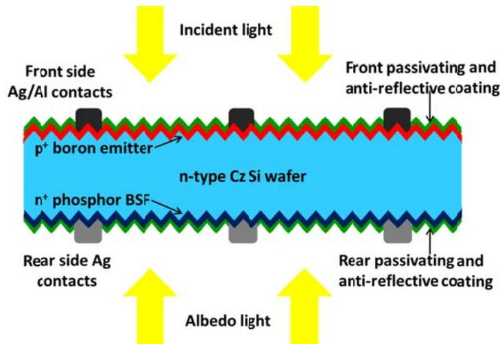
Figure 1. Cross section of the ECN n-Pasha cell. Yingli's PANDA cells are based on this structure.
