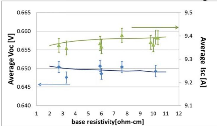
Figure 3: Average  $V_{oc}$  and  $I_{sc}$  as function of base doping of the n-Cz material. The error bars indicate the variation (max-min) within the IV results. The solid lines are PC1D fits using fixed values for all parameters except the base resistivity.
