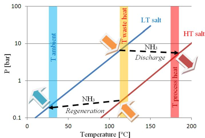
**Figure 2: Thermodynamic cycle of the heat-driven heat pump type II configuration.**
