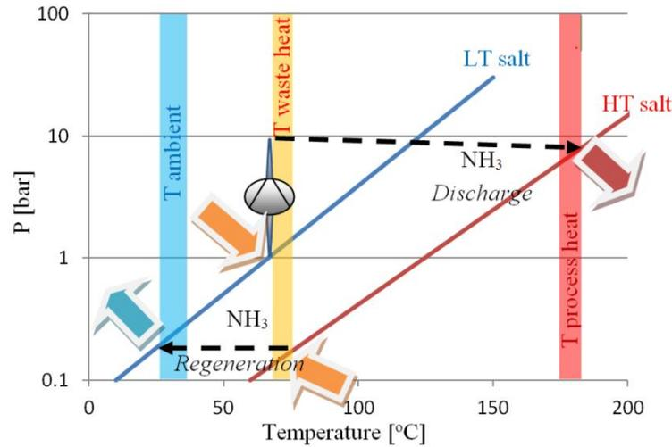
**Figure 3: Thermodynamic cycle of the hybrid heat pump type II configuration.**
