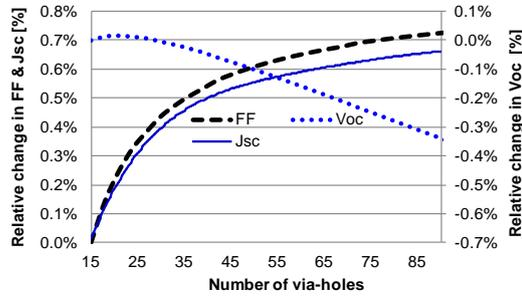
**Fig. 2** Calculated relative FF,  $I_{sc}$  and  $V_{oc}$  changes as a function of the number of via-holes for n-MWT cells.
