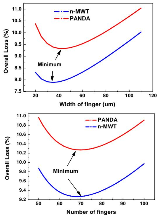
**Figure 2:** Calculated relationships between front finger pattern and the overall-loss, for both n-MWT and PANDA. (Top: width of fingers; Bottom: number of fingers)
