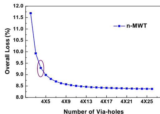
**Figure 3:** Influence of n-MWT via-hole number on the overall loss.
