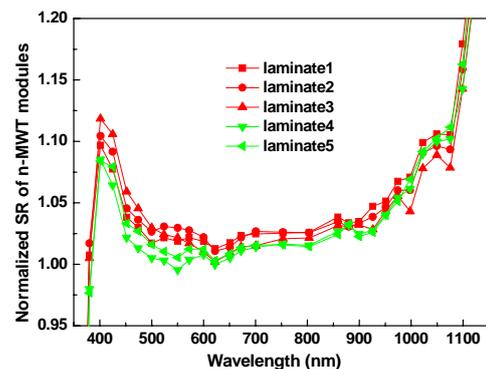
**Figure 5:** Influence of backfoil on SR of n-MWT laminates. (The green data from Foil-A; the red data is from Foil-B)
