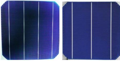
**Figure 1:** Images of the front side for an n-MWT cell (left) and a normal PANDA cell (right).
