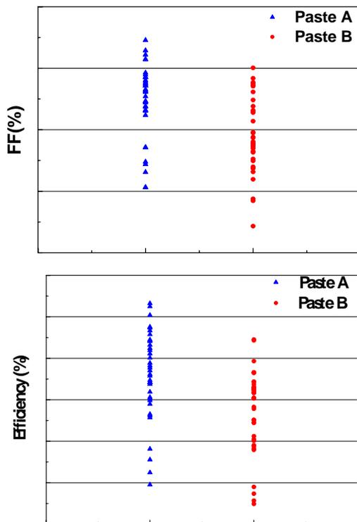
**Figure 4:** Relative distribution of FF (top, grid line separation is 0.5% of FF) and Efficiency (bottom, grid line separation is 0.1% of efficiency) as a function of Plug pastes
