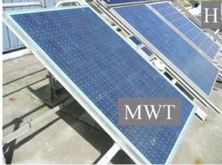
**Figure 2:** Part of IV tracing system at ECN with 60 cell MWT module (left) and 54 cell H-pattern module (right).
