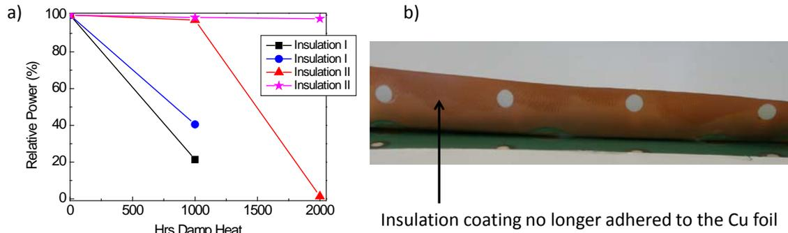
Figure 3. a) relative power of MWT back contact modules comprised of EVA and back sheet foil with insulation coating, as a function of damp heat exposure, up to 2000 hrs (2xIEC) b) photographic image of an MWT module opened after 2000 hrs of damp heat testing. The insulation coating is no longer attached to the Cu foil.
