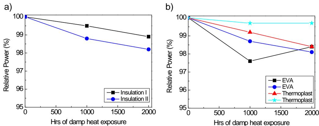
Figure 4. Relative power of MWT modules as a function of damp heat exposure. a) MWT back contact modules comprised of thermoplastic and back sheet foil with insulation coating b) MWT back contact modules comprised of either EVA or thermoplastic and back sheet foil without insulation coating.
