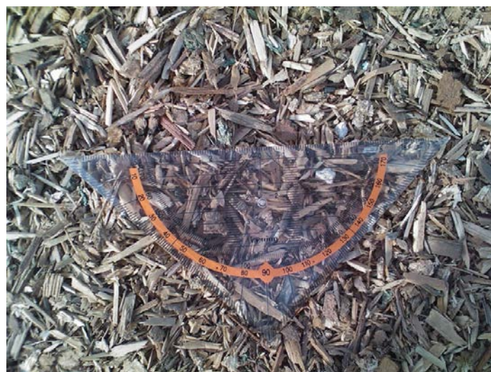
FIGURE 5: DEMOLITION WOOD B AS TESTED IN THE MILENA PILOT PLANT.
