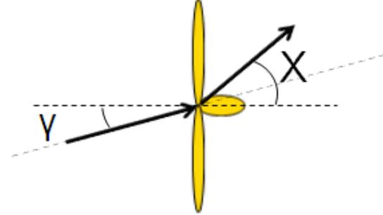
Figure 2: Yaw misalignment and wake skew angle. The arrows indicate the wind and wake directions.
