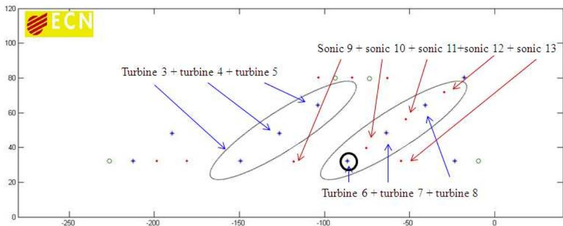
Figure 1: Layout of the scaled wind farm. Turbines 3, 4 and 5 form the reference row (Row 1) and turbines 6, 7 and 8 the CW row (Row 2). Turbine 6 is misaligned.
