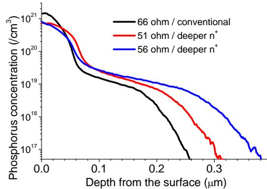
**Fig. 1** Phosphorus doping profiles of 51 and 56  $\Omega/\text{sq.}$  emitters with deeper n<sup>+</sup> and lower  $N_p$  in the n<sup>++</sup>, and 66  $\Omega/\text{sq.}$  emitter made of conventional process.
