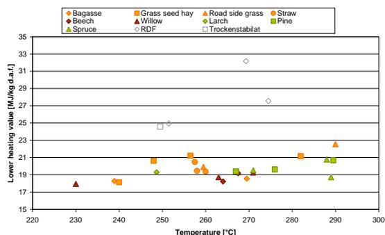
**Figure 7:** LHV of the materials produced by torrefaction at different temperatures.
