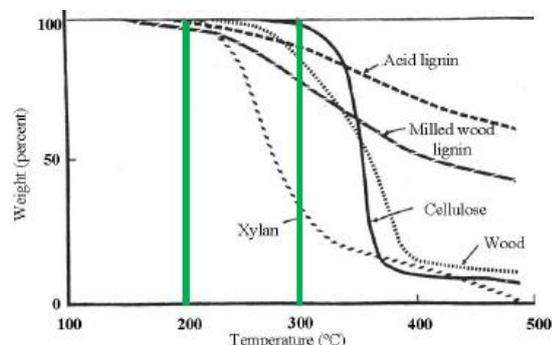
**Figure 2:** Thermogravimetry of cotton wood and its constituents [9]
