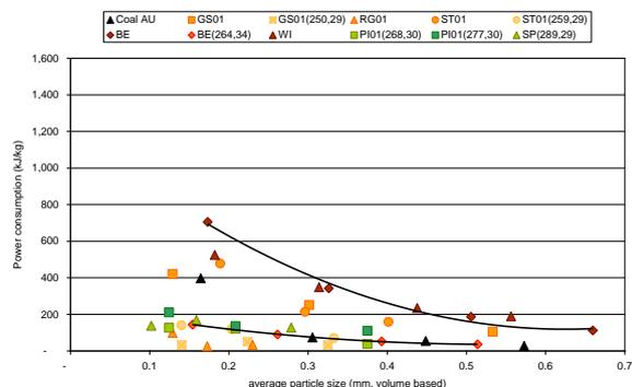
**Figure 4:** Power consumption as a function of final particle size (torrefaction conditions in brackets, temperature in °C, residence time in minutes)
