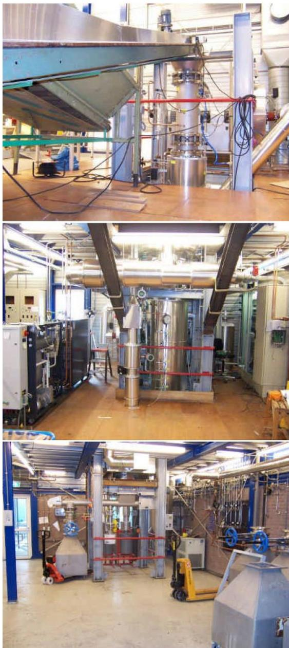
**Figure 6:** Top, middle and bottom section of the PATRIG torrefaction pilot plant
