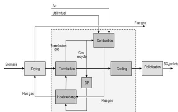
**Figure 4:** Process flow diagram of BO<sub>2</sub>-technology.
