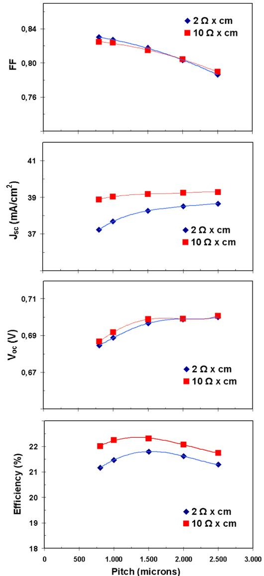
**Figure 5. 2D simulations results showing the variation versus pitch of (a) Fill factor (FF), (b) Short circuit current ( $J_{sc}$ ), (c) Open circuit voltage ( $V_{oc}$ ) and (d) efficiency for base resistivities of 2  $\Omega$  x cm and 10  $\Omega$  x cm, respectively.**
