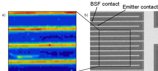
**Figure 6. (a) LBIC measurement and (b) optical image showing difference between losses on BSF and Emitter contacts.**
