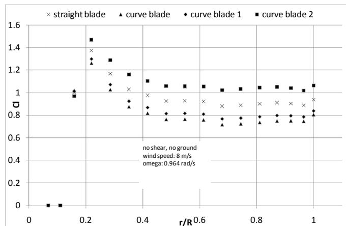
Figure 2 Lift coefficient distribution along the blade. Comparison between the geometries.
