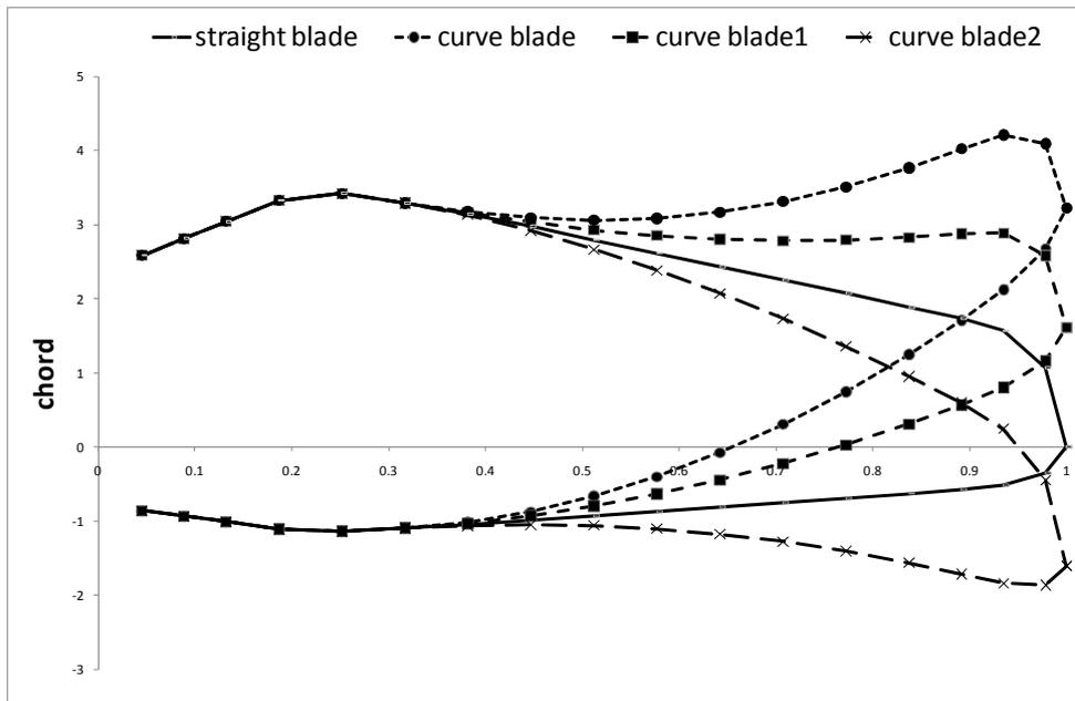
Figure 1 Blade geometries used during the parametric analysis.
