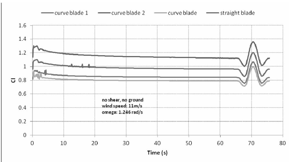
Figure 4 Time evolution of local lift coefficient at 92% of the blade.
