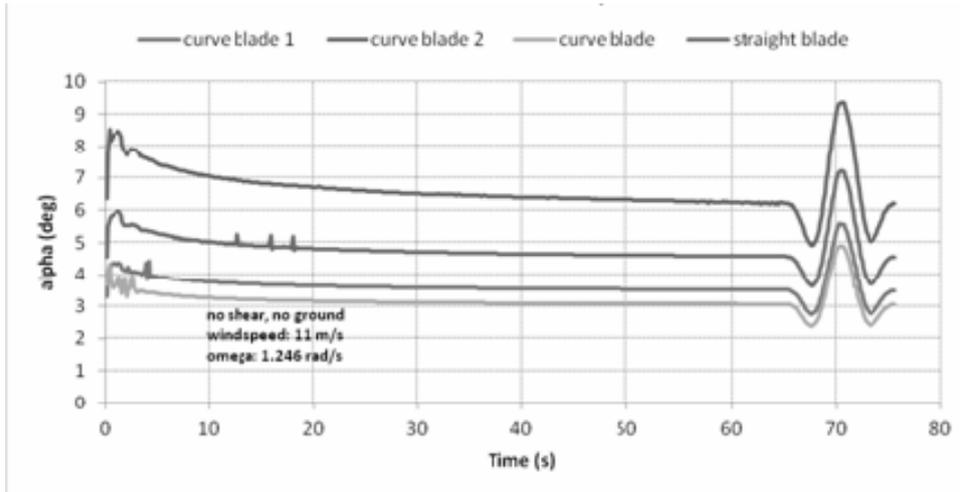
Figure 3 Time evolution of local angle of attack at 92% of the blade.
