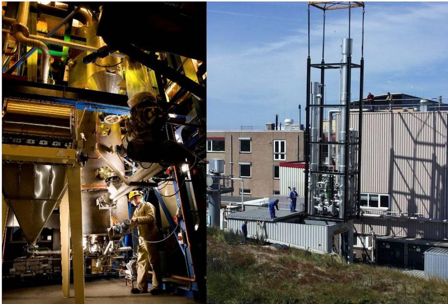
Figure 4: Pilot-scale MILENA gasifier (left) and installation of the OLGA pilot-scale gas cleaning (right).
