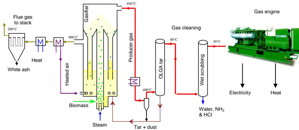
Figure 2: Basic layout of MILENA Bio-CHP plant.
