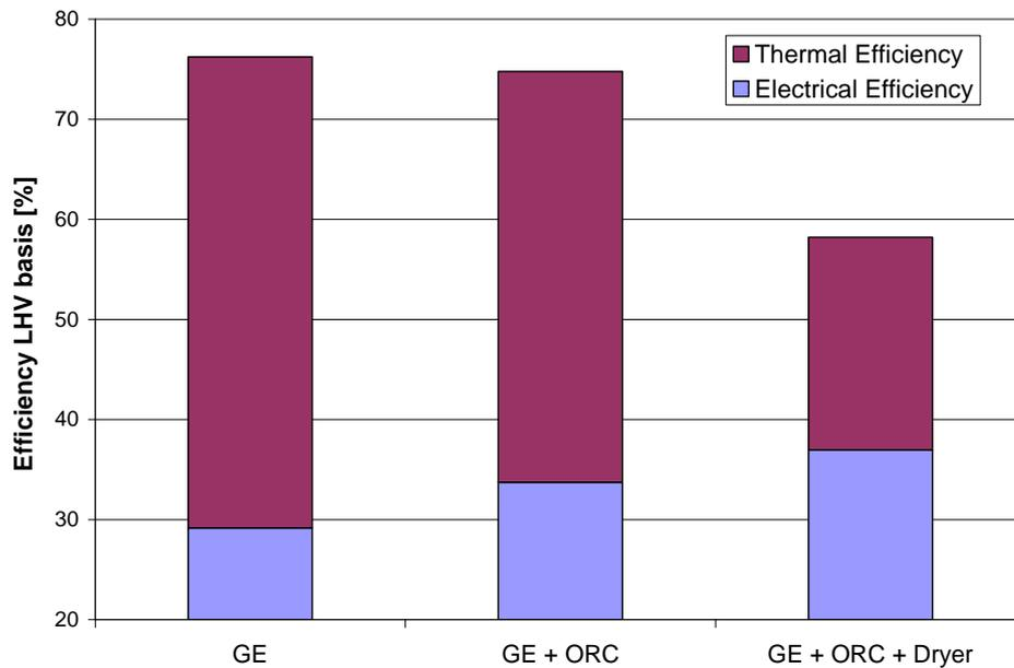
Figure 3: Calculated efficiencies of MILENA Bio-CHP configurations; GE: Gas Engine, ORC: Organic Rankine Cycle.
