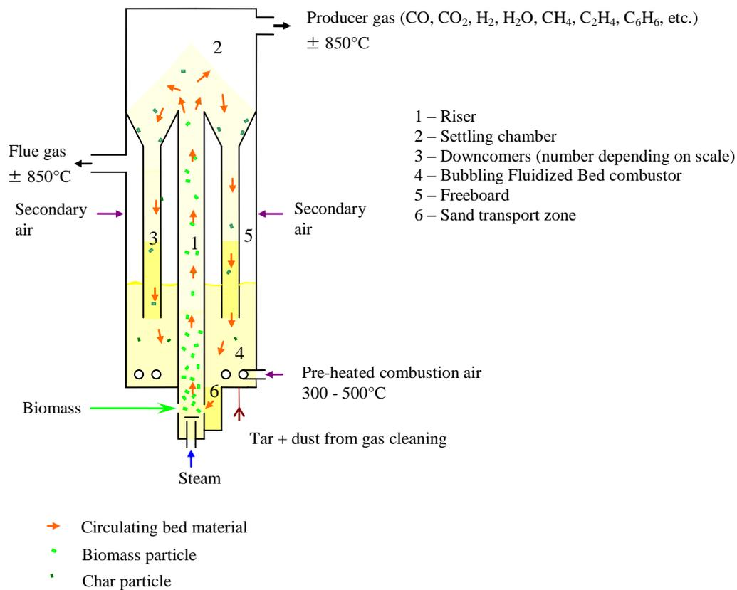
Figure 1: Simplified scheme of MILENA gasifier.
