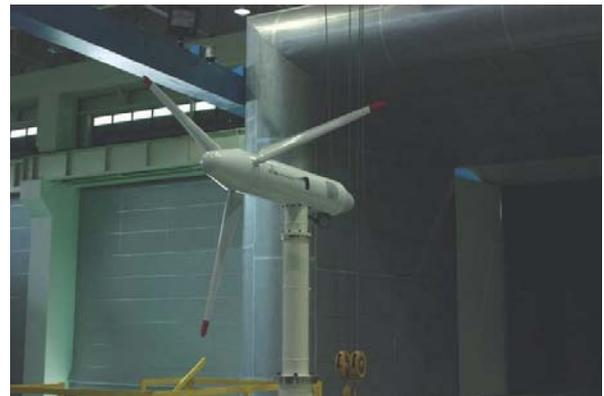
Figure 3: KARI wind tunnel with scaled down model of Mexico rotor, compare with figure 1
