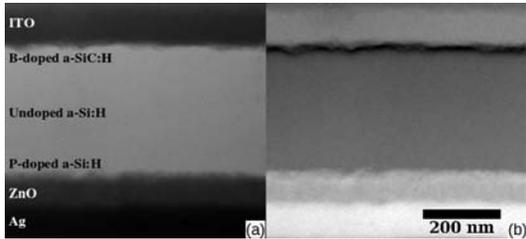
**Figure 2:** (a) Bright field and (b) thickness over lambda TEM image of an a-Si solar cell prepared using focus-ion-beam milling.
