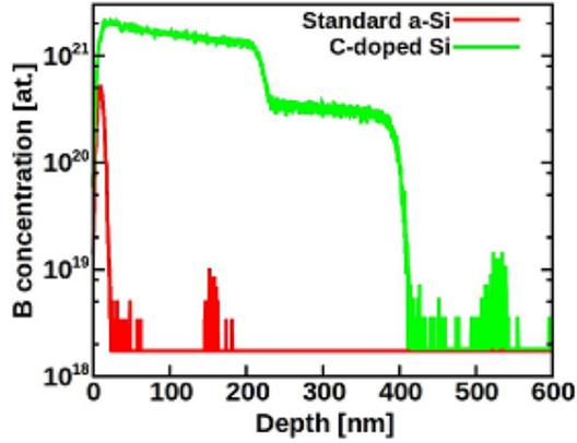
**Figure 1:** Boron concentration profiles by SIMS measurements of a n-i-p a-Si solar cell (red) and of the SiC test samples with three levels of p-type doping (green).
