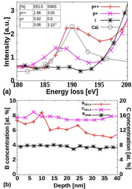
**Figure 6:** (a) Background subtracted core-loss EELS of the SiC stack with three different B concentrations. Insert: estimation of the B concentration calculated from the area below the curve. SIMS values have been obtained on the same sample. (b) B and C concentration profiles measured by TEM-EELS with a 5 nm probe. The B concentration profile measured by SIMS is shown for comparison.
