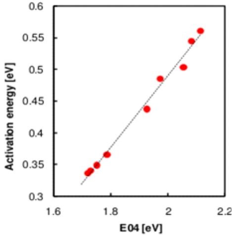
**Figure 4:** Relation between  $E_{act}$  and  $E_{04}$  data, obtained by varying the  $B_2H_6$  and  $CH_4$  flow rates. The dashed line is a linear fit to the data.
