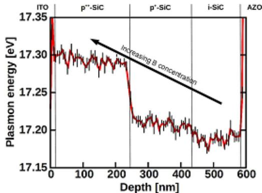
**Figure 7:** Plasmon energy as a function of depth relative to the ITO/p<sup>++</sup>-SiC interface. The dashed lines represent the locations of the interfaces.
