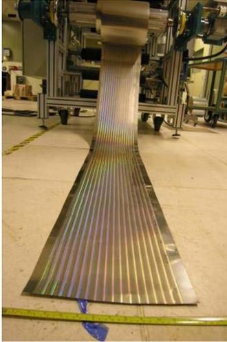
**Figure 8:** Periodic texture on steel foil made by roll-to-roll nano-imprinting.
