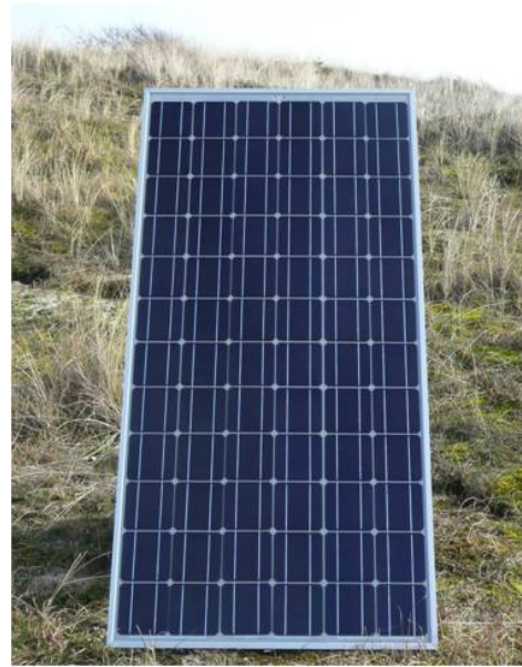
Figure 7: Hetero-junction module with 72 cells, manufactured at the ECN tabber stringer using conductive adhesive.
