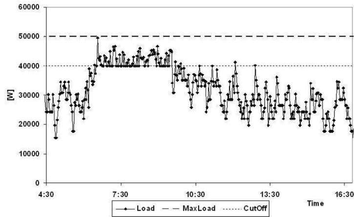
**Fig. 3.** Peak load reduction achieved at a substation on a cold morning for 20 dwellings. The transformer station operates at a maximum permitted load which is 30% of maximum load without control.
