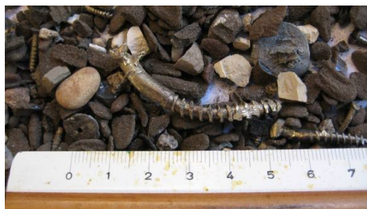
Figure 6: Bottom ash discharge from riser
