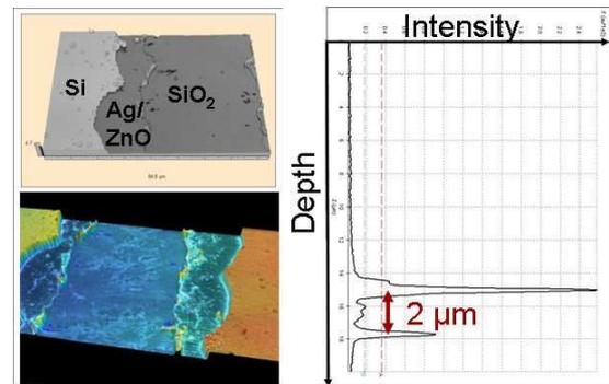
**Figure 13.** Confocal microscopy analysis of the P1 laser scribe.
