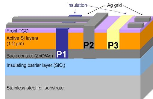
Figure 6. Thin-film silicon PV Module concept on electrically insulated steel foil substrate.
