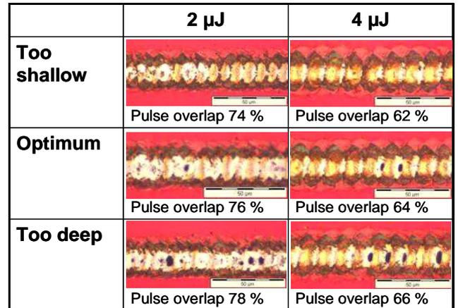
**Figure 8.** Pulse energy / pulse overlap combinations to achieve P2 scribes with the UV ns laser.
