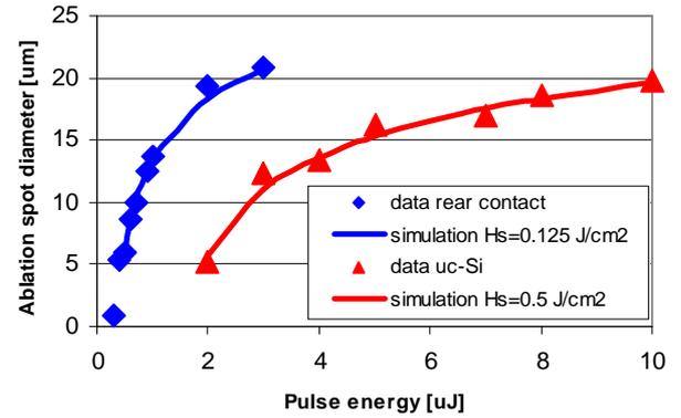
**Figure 7.** Ablation diameter versus pulse energy for the back contact and the  $\mu$ c-Si layer. Fitting of these curves yields the ablation thresholds of the corresponding layers for the 355 nm laser.
