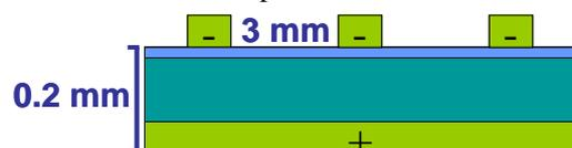
Figure 1. Standard 'H-pattern' solar cell.
