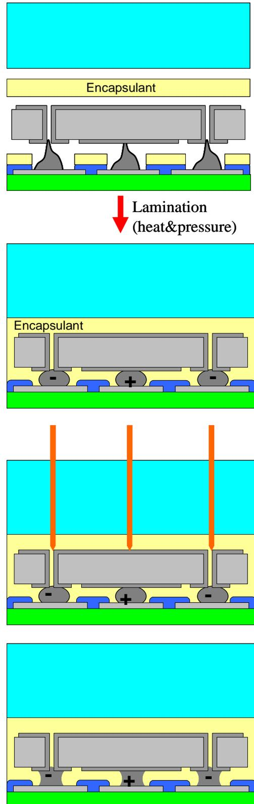
**Figure 5.** Process sequence for in-laminate laser soldering.
