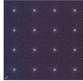
**Figure 3.** Typical metallization wrap-through solar cell with 16 vias and grid pattern optimized by ECN\*.
