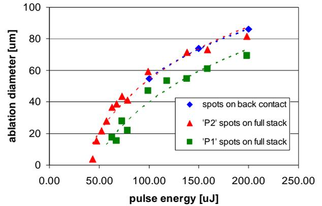
**Figure 12.** Diameter of ablation versus pulse energy with 1064 nm laser.
