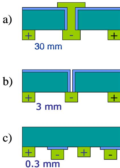
**Figure 2.** Next generations of crystalline silicon solar cells: a) metallization wrap-through (MWT), b) emitter wrap-through (EWT) and c) interdigitated back contacted cells (IBC). The typical dimensions of a ‘unit cell’, i.e. distance between positive and negative electrodes, is indicated.
