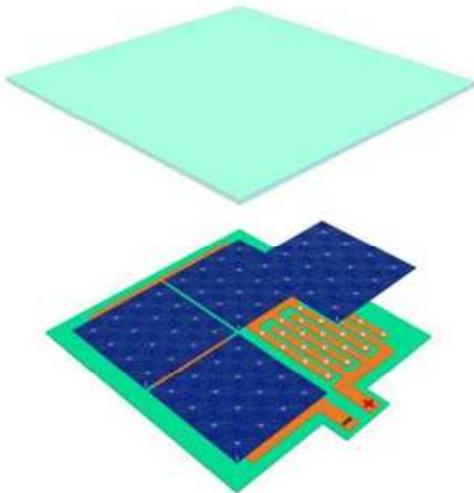
**Figure 4.** Module concept for back-contacted solar cells with low-resistive pattern in backsheet foil, and compatibility with pick-and place technology for cell alignment.\*
