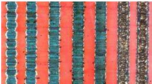
**Figure 10.** P1 scribes obtained with a 1064 nm ns pulsed laser. From left to right the spot overlap was increased
