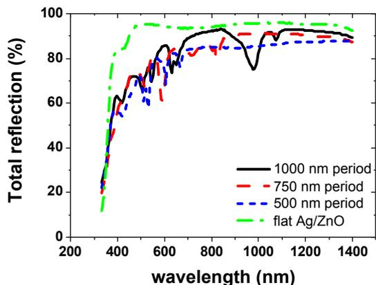
**Figure 5:** Total reflection spectrum of three differently textured Ag/ZnO back contact diffraction gratings and a flat reference back contact.
