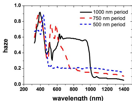
**Figure 6:** Haze of three differently textured Ag/ZnO back contact diffraction gratings.
