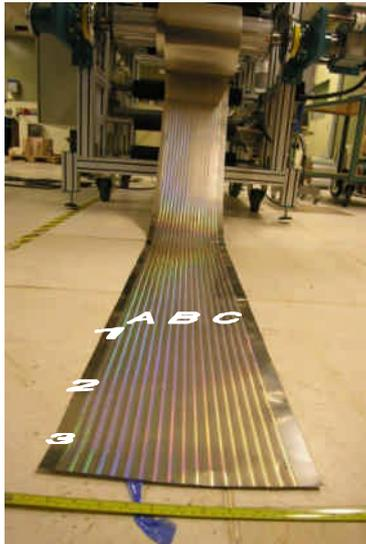
**Figure 3:** Photograph of a roll-to-roll nanotextured lacquer on steel foil substrate. The numbers and characters correspond to the matrix of SEM images in Figure 4.
