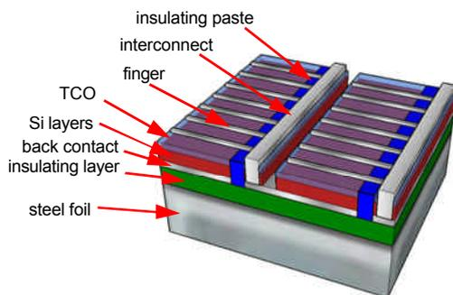
**Figure 1:** ECN's thin film Si solar cell and module concept.
