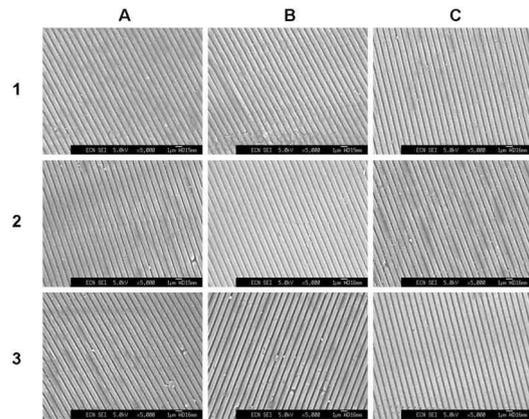
**Figure 4:** SEM images on the nine locations depicted in Figure 3, showing the nanotexture in the lacquer on steel foil.
