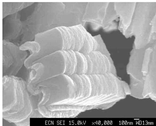
**Figure 7:** SEM cross section of a fragment of an a-Si:H solar cell on a 500 nm grating back contact.
