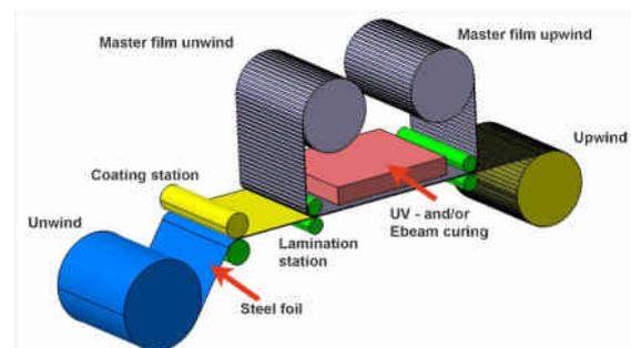
**Figure 2:** Schematic showing the principle of the contact imprint technology.
