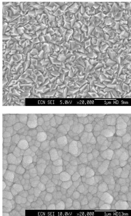
Figure 3: SEM picture of an Asahi U texture (top) and the ITO surface of a nip solar cell grown on Asahi-U glass substrate coated with a sputtered Ag/ZnO back contact (bottom).
