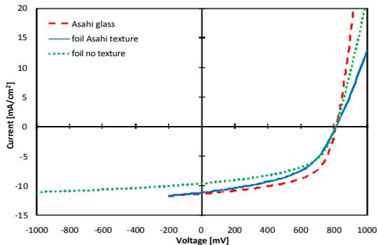
Figure 5: JV-curve of nip solar cell deposited on steel foil coated with Asahi-textured barrier layer and Ag/ZnO back contact compared with nip solar cell deposited on Asahi glass (dashed, red). Flexible cells with Asahi-textured barrier layer and flat barrier layer are shown, respectively as solid blue and dotted green lines.
