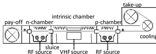
**Figure 1:** Cross-section through the Flexicoat300 roll-to-roll PECVD system.
