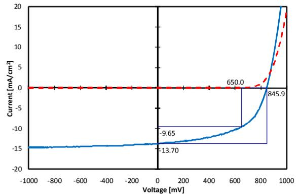
Figure 2: JV-curve of nip solar cell on a rigid substrate: Asahi U-type glass coated with a sputtered Ag/ZnO back contact.
