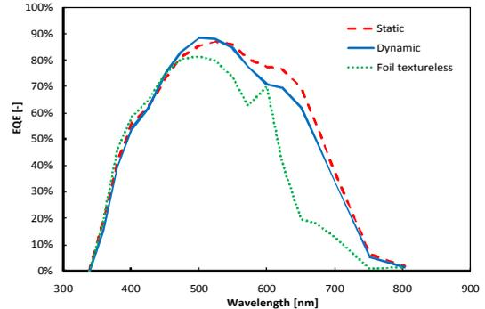
Figure 6: EQE curves of the presented solar cells: step-roll (dashed, red), in-line on rigid substrate (solid, blue) and in-line on flexible, texture-less substrate (dotted, green).
