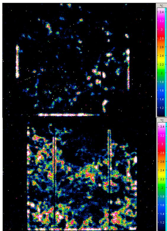
**Figure 7:** Lock-in Thermographs at 2V reverse bias for the Fe50 (top) and Fe200 (bottom) ingots at 23% and 32% ingot height, respectively. The pattern corresponds to microscope observations of the filament distribution on neighbouring wafers.
