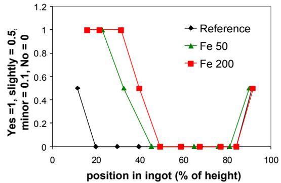
**Figure 5:** qualitative analysis of filament distribution over the ingot by dark lines in optical microscope (1 = filaments on more than 30% of the wafer area, 0.5 = more than 10 grains with filaments but less than 30% of the wafer area, 0.1 = less than 10 grains with filaments, 0 = no dark lines).
