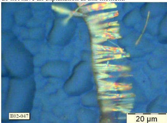
**Figure 2:** Higher magnification image of a “dark colored boundary”. This image is taken on a chemically etched wafer from a Cr contaminated ingot.
