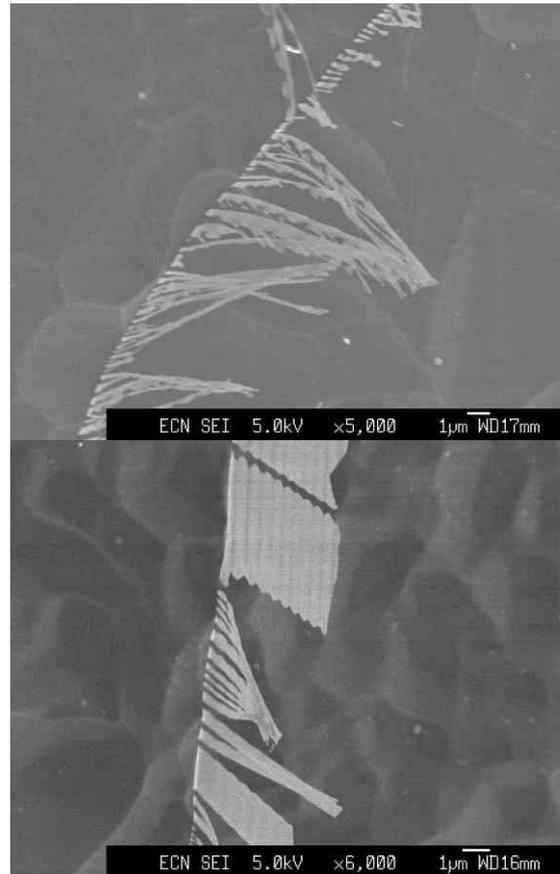
**Figure 3:** SEM observations of silicon nitride sheets and filaments sticking out of the grain boundaries. Very peculiar is the “waviness” of these sheets, which seems to be periodic.
