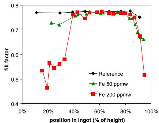
**Figure 6:** Fill factor distribution of solar cells as a function of ingot position. The two Fe contaminated ingots display a distinct drop in FF in the bottom region up to about 35% ingot height. The FF reduction in the bottom is considerably larger for the ingot with 200 ppmw of Fe than for the ingot with 50 ppmw of Fe.
