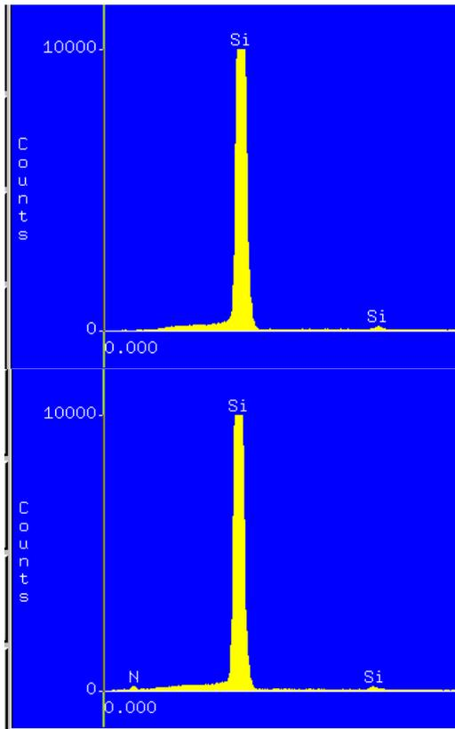
**Figure 4:** Top: EDX measurement on bare silicon surface. Bottom: EDX measurement on silicon nitride sheet (with silicon surface background). Evidently, the sheet contains nitrogen.
