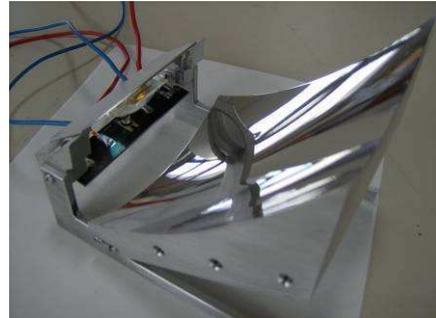
**Figure 5:** CPower optimized prototype of a single unit (or sub-module) of the module
