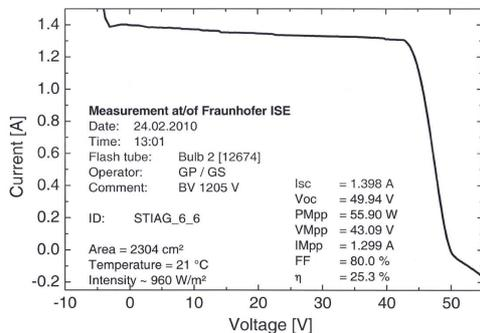
**Figure 4:** Solartec optimized module IV curve. Active area 0.23 m<sup>2</sup>, total area 0.26 m<sup>2</sup>
