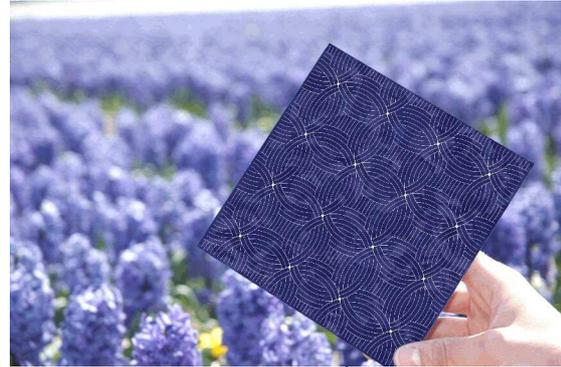
Figure 1: Photograph of a 243 cm<sup>2</sup> back-contacted MWT cell.
