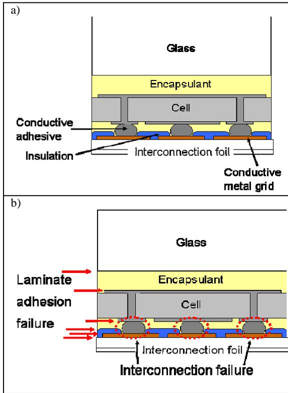
**Figure 2:** a) Schematic cross section of a back contact module. b) Indication of positions where failure could start to occur. Red arrows indicate points where adhesion of layers is relevant, the dotted circles indicate where interconnection failure could start.
