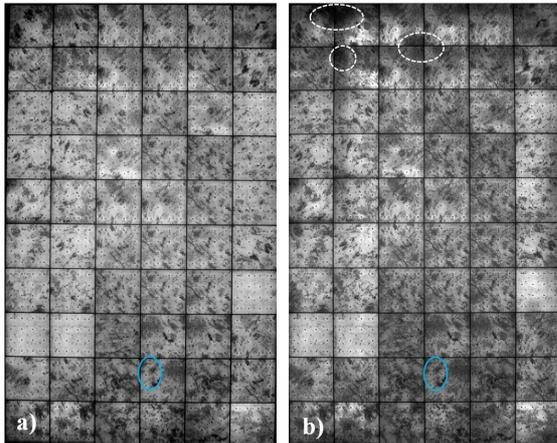
**Figure 4:** EL images of module M5, before (a) and after (b) 300 thermal cycles. The blue ellipse indicates a cracked cell. The white ellipses indicate regions where the EL intensity has dropped upon thermal cycling. Images were taken with 8A forward bias.
