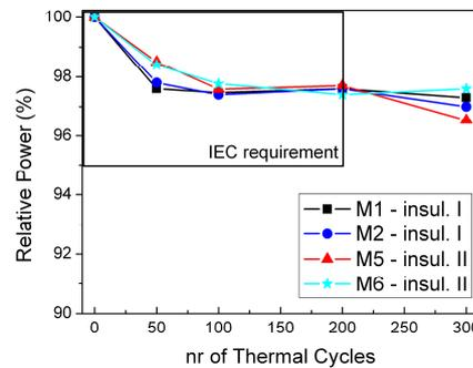
**Figure 3:** Relative power after exposure to 300 thermal cycles for modules M1, M2, M5 and M6.
