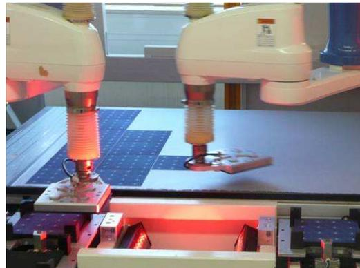
**Figure 1:** Cell pick and place in the back contact module manufacturing process.
