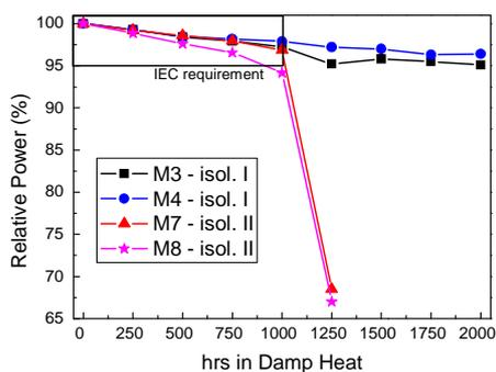
**Figure 5:** Relative power after 2000 hrs of damp heat exposure for modules M3, M4, and after 1250 hrs of damp heat exposure for modules M7 and M8.
