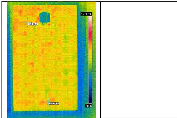
**Figure 6:** IR images of a) M3 after 2000 hrs damp heat exposure. Temperature differences are less than 2°C, and b) M7 after 1000 hrs damp heat exposure (just before string failure started to occur). Temperatures measured range from 24.7°C (green) to 40.3°C (bright red).
