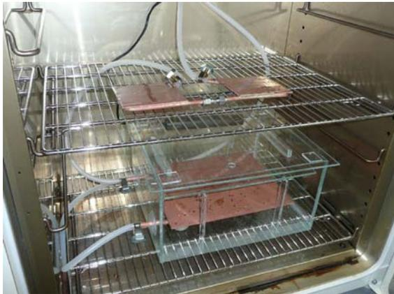
**Figure 3:** Photo of the ATF showing the glass box with the different sample holders
