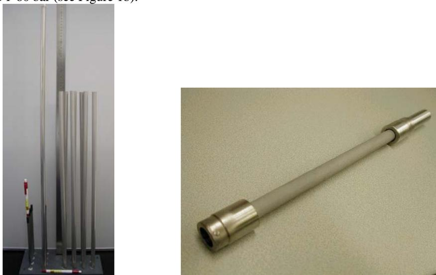
Figure 1. Set of PdAg membrane tubes with a length of 0.6 meter (a) and a membrane with the low cost carbon compression sealing (b).
