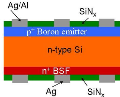
*Figure 3 - Schematic cross-section of the n-type solar cell.*
