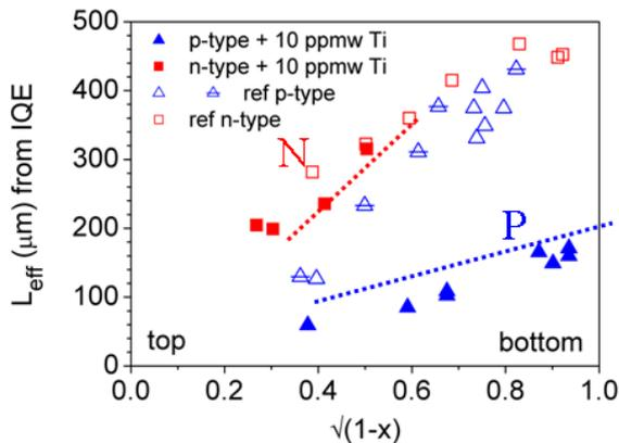
**Figure 1 - Comparison of  $L_{eff}$  of n-type and p-type mc-Si ingots contaminated with Ti as a function of ingot position.**
