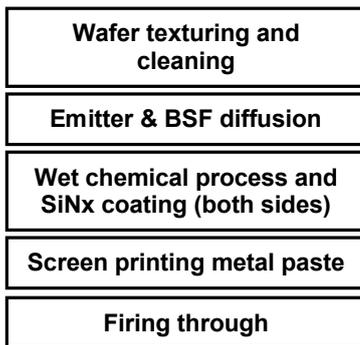
*Figure 2 - Major process steps for making industrial screen printed n-type solar cells.*
