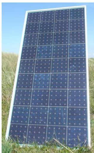
**Figure 1:** The finished module showing the characteristic cell pattern. All of the conductive back-sheet is within the active area of the cells. There is no need for bussing at the top and bottom of the module resulting in increased module efficiency when compared with H-pattern modules.
