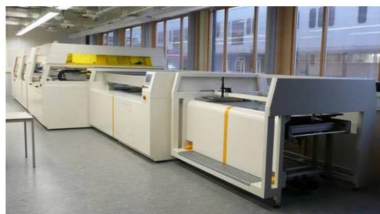
**Figure 2:** The module pilot line at ECN. The module building starts at station 1 at the front of the picture with positioning of the foil on the carrier plate
