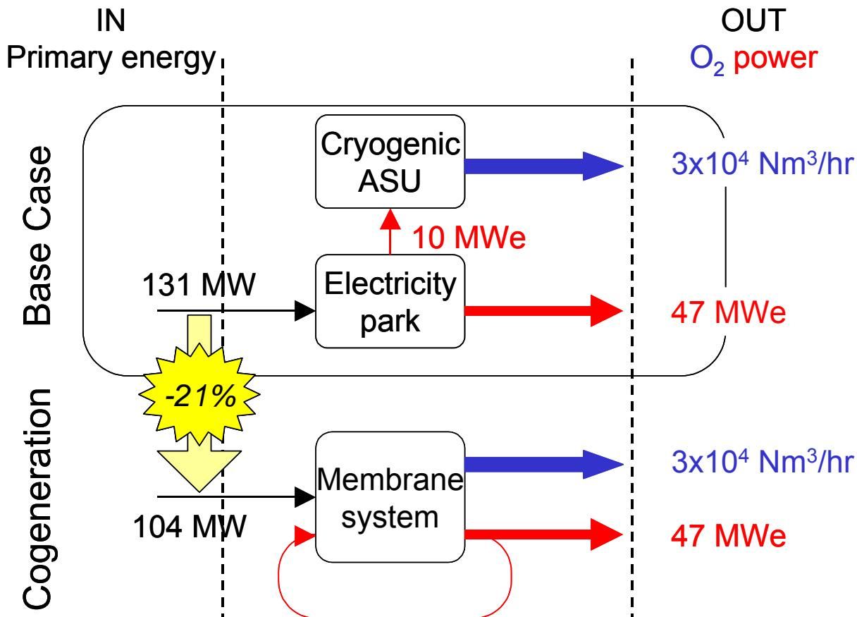
Reduction of energy use when combined with electric power production
