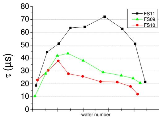
Figure 2: Lifetime of ingots FS9, FS10 and FS11.
