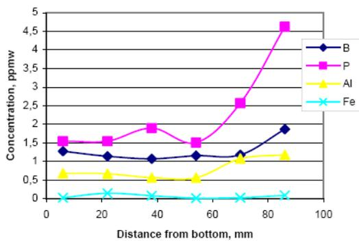
Figure 3: Chemical concentration of the B, P, Al and Fe for ingot FS1 as measured by GDMS.
