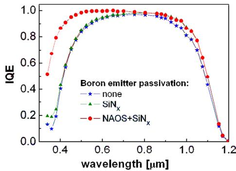
Figure 7: Internal quantum efficiency of the n-type solar cells measured for different passivation methods for boron emitter.
