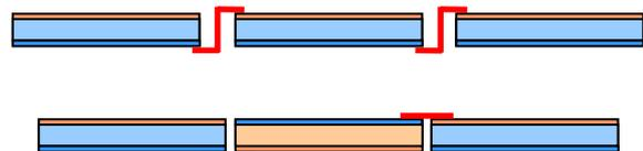
Figure 6: Interconnection of p-type solar cells in a standard module (top) and innovative alternate interconnection of p- and n-type solar cells in a pn-module (bottom) (pending patent by ISC Konstanz).
