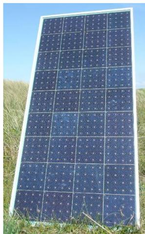
**Figure 9:** The world record module, with 16.4% efficiency on an aperture area of 8904 cm<sup>2</sup>.
