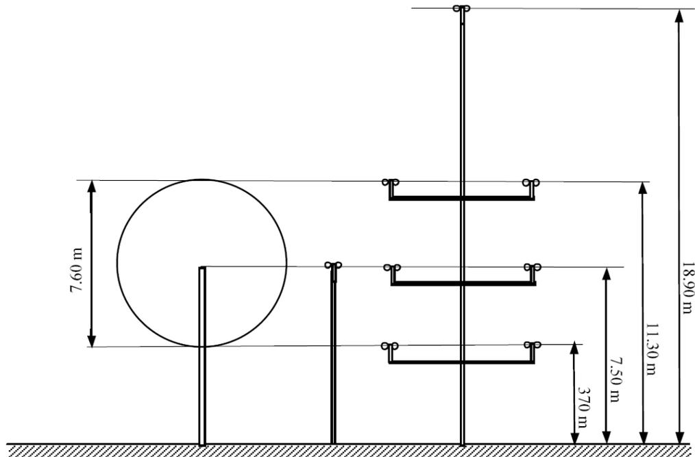
Figure 1. Scales in the ECN scale wind farm.
