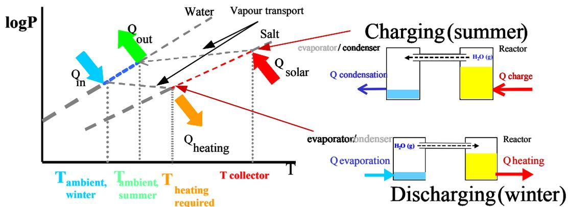
Figure 3: TCM system as an absorption heat pump
