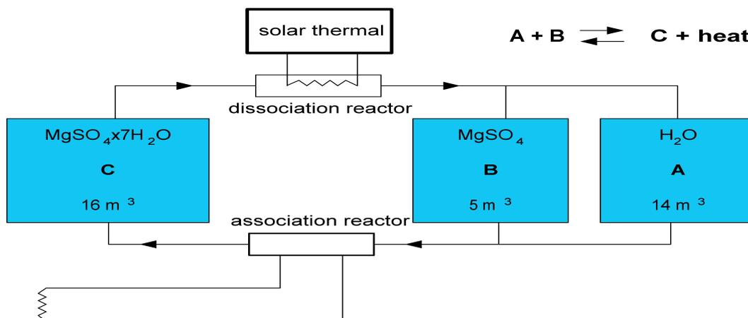
**Figure 2: TCM system for seasonal storage for a space heating system (heating demand 44 GJ).**
