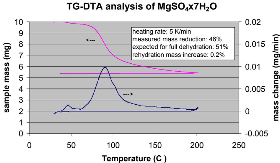
**Figure 1: TG-experiments on  $\text{MgSO}_4 \cdot 7\text{H}_2\text{O}$  (high heating rate)**
