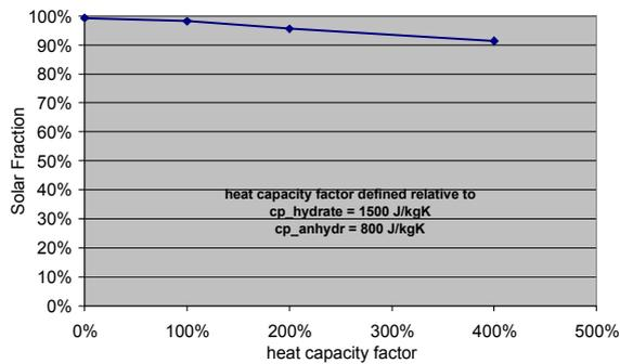
Figure 4: Effect of TCM heat capacity on solar fraction
