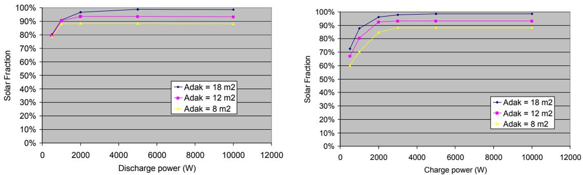
Figure 5: Effect of charge power and discharge power on solar fraction
