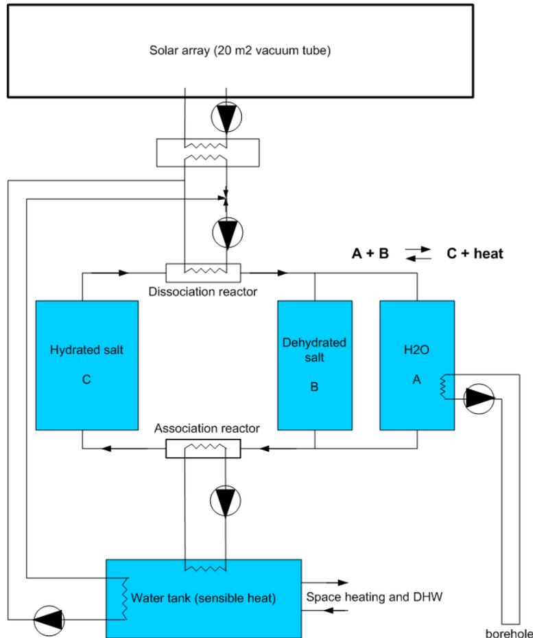
**Figure 1: Lay-out of the investigated system.**
