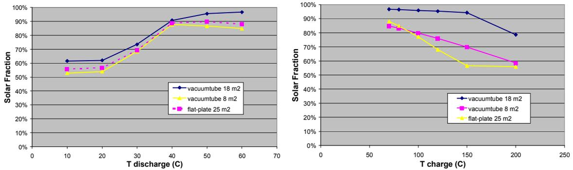
Figure 3: Effect of charge temperature and discharge temperature on solar fraction.
