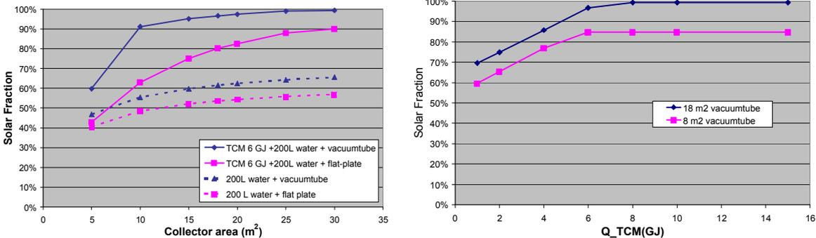
**Figure 2: Effect of collector area and TCM storage capacity on solar fraction**
