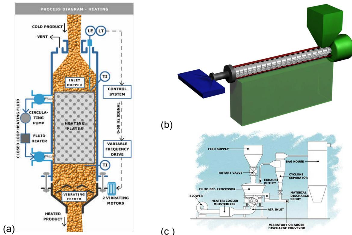
Figure 6: reactor types (a) bulkflow ([www.bulkflow.com](http://www.bulkflow.com)), (b) screw reactor for plastics extrusion ([wikipedia](http://wikipedia)), (c) fluidized bed reactor ([www.kason.com](http://www.kason.com))
