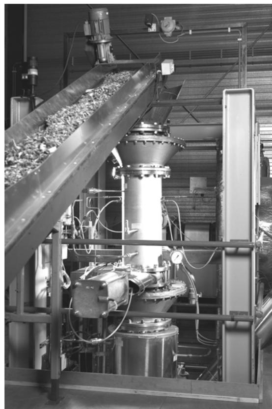
**Figure 6:** Biomass being fed to the top section of the pilot plant (Photo Jasper Lensselink)
