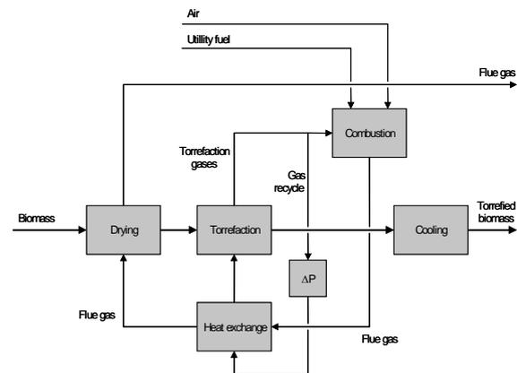
**Figure 4:** Process flow diagram of BO<sub>2</sub>-technology. Only the integrated drying-torrefaction part of the process is shown (not size reduction and pelletisation).
