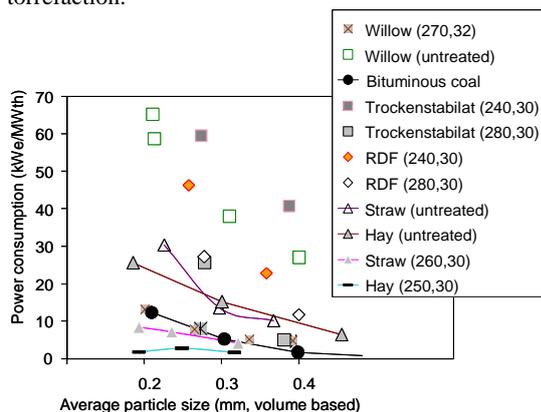
**Figure 3:** Grinding behaviour of a range of feedstocks, including agricultural residues and waste derived fuels
