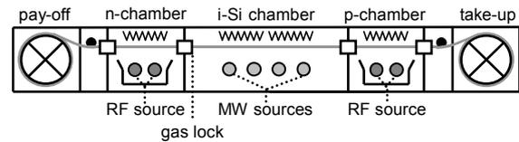
**Figure 1:** Cross-section through the FLEXICOAT300 roll-to-roll coater. Both RF sources, in the n- and p-chamber, contain two parallel linear electrodes, whereas the four MW sources have one antenna each in a quartz tube.
