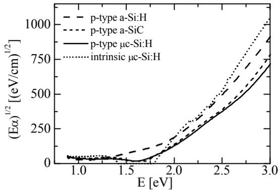
**Figure 5:** Tauc plot,  $(E\alpha)^{1/2}$  as a function of  $E$  [6], of the samples shown in Table 1. The a-Si:H sample has an order of magnitude higher absorption compared with the other three samples.
