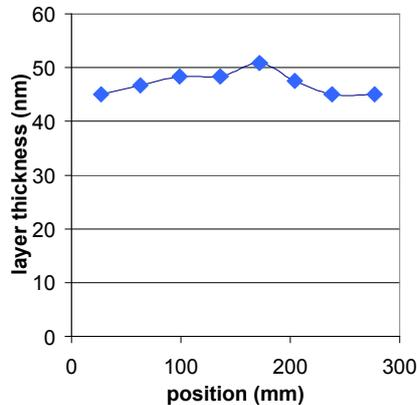
**Figure 2:** Thickness variation of an a-Si layer grown with the linear RF source. The variation is less than 4%.
