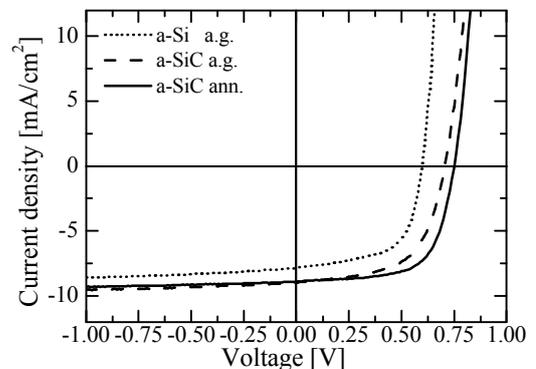
**Figure 7:** I-V curves for a-Si solar cells with an a-Si:H window layer (as grown: dotted), an a-SiC window layer (as grown: dashed) and the a-SiC solar cell after annealing (solid).
