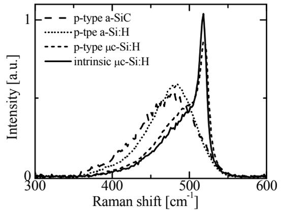
**Figure 6:** Raman spectra of the samples shown in Table I. The sharp peak at  $\sim 518 \text{ cm}^{-1}$  is due to the TO mode in crystalline Si, the much broader peak at  $480 \text{ cm}^{-1}$  is due to the TO mode in a-Si:H. Layer thicknesses are about  $\sim 200 \text{ nm}$  and given in Table I.
