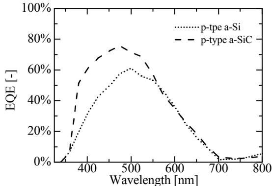
**Figure 8:** EQE curves for the two solar cells shown in Figure 7, after annealing. Solid and dashed lines represent the solar cells with the a-Si:H and a-SiC:H p-type window layers, respectively.
