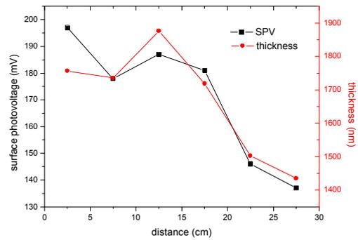
**Figure 3:** SPV results and thickness data for an inhomogeneous layer.
