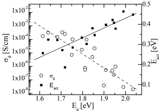
**Figure 4:**  $\sigma_d$  (left axis, open circles) and  $E_{act}$  (right axis, solid squares) as a function of  $E_g$ . The lines are linear fits: increasing  $\text{CH}_4$  flow or decreasing  $\text{B}_2\text{H}_6$  flow results in a higher  $E_g$ , but a lower  $\sigma_d$  and higher  $E_{act}$ .
