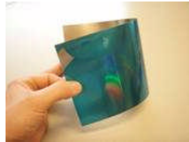
Figure 3. Regular grating structure embossed into the insulating barrier layer, efficiently dispersing the light. The observed rainbow colors are due to dispersion, demonstrating the successful replication of the master into the insulating layer
