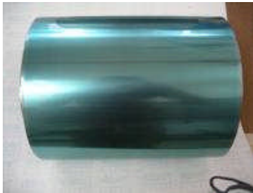
Figure 2. The 30 cm wide steel foil with an insulating \text{SiO}_x barrier layer applied by roll-coating.
