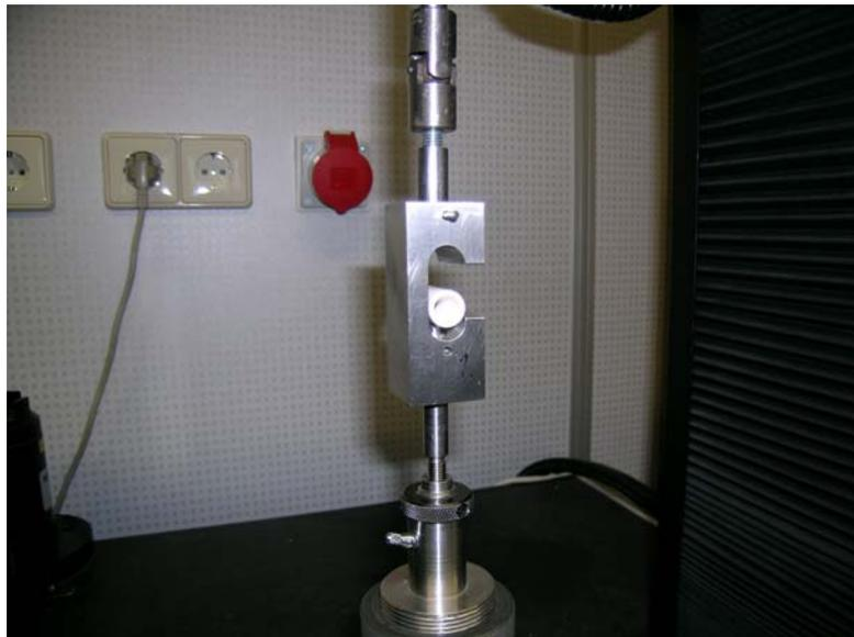
Figure 3.2 *Tensile test set up as developed at ECN*
