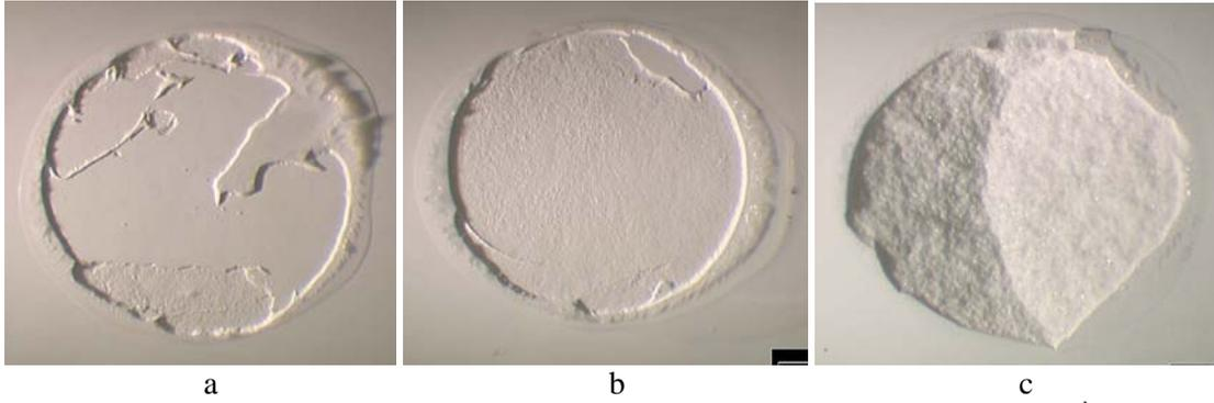
Figure 3.4 *Fractography of the fractures surfaces: a, 1100°C - interface 1<sup>st</sup> and 2<sup>nd</sup> layer, b = 1200°C – interface support tube and 1<sup>st</sup> layer, c = 1300°C – bulk material support tube*
