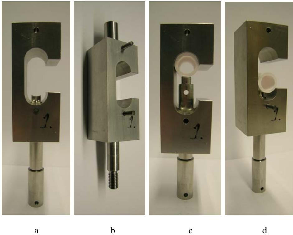
Figure 3.1 *Test tool and holder for tensile testing of tubular samples*
