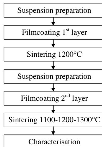
Figure 2.1 *Processing flow sheet for standard ECN support system*
