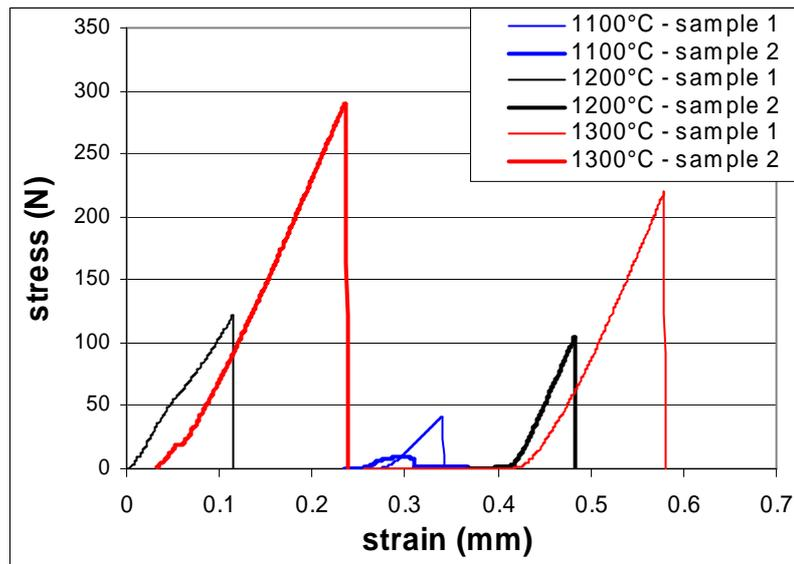
Figure 3.3 *Stress-strain diagram for the asymmetric supports sintered at 1100, 1200 and 1300°C.*
