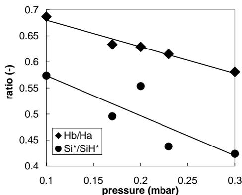
**Figure 8:** Ratio of  $H\beta/H\alpha$  and  $Si^*/SiH^*$  emission intensities versus operating pressure for  $H_2/SiH_4$  plasma with a flow ratio of 99. The lines are linear fits to the data.
