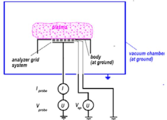
**Figure 4:** Principle of retarding field analyzer.
