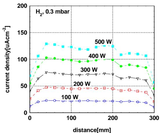
**Figure 6:** Ion density profile of a hydrogen plasma generated by the linear RF source at 0.3 mbar.
