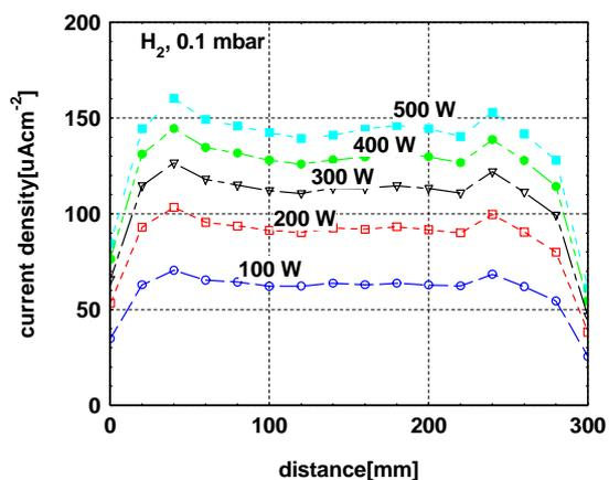
**Figure 5:** Ion density profile of hydrogen plasma generated by the linear RF source at 0.1 mbar as a function of RF power.
