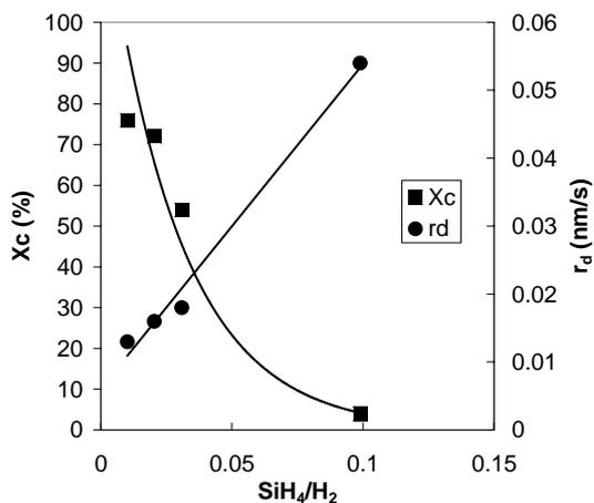
**Figure 10:** Crystal fractions ( $X_c$ ) and deposition rates ( $r_d$ ) for intrinsic layers grown at various SiH<sub>4</sub>/H<sub>2</sub> ratio's. The trend lines serve as a guide to the eye.
