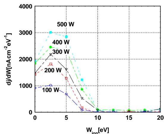
**Figure 7:** Ion energy distribution of the linear radio frequency plasma source versus applied RF-power at 0.1 mbar hydrogen.
