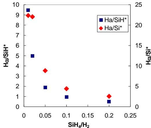
**Figure 9:** Ratios of H $\alpha$ /SiH and H $\alpha$ /Si\* emission intensities as a function of SiH<sub>4</sub>/H<sub>2</sub> gas flow ratio.
