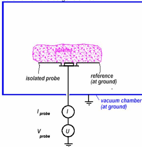
**Figure 3:** Principle of the Langmuir probe.
