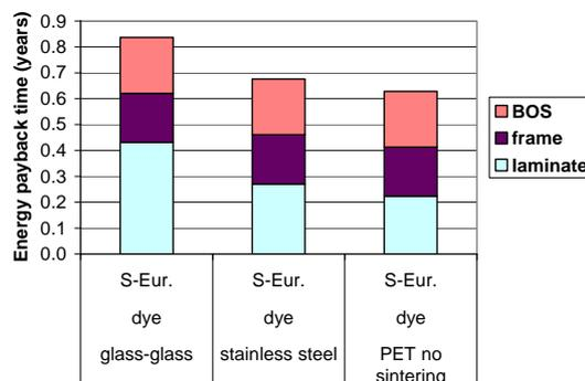
**Figure 2:** Energy payback time in Southern Europe for PV systems using DSC modules with different substrates (8% module efficiency).
