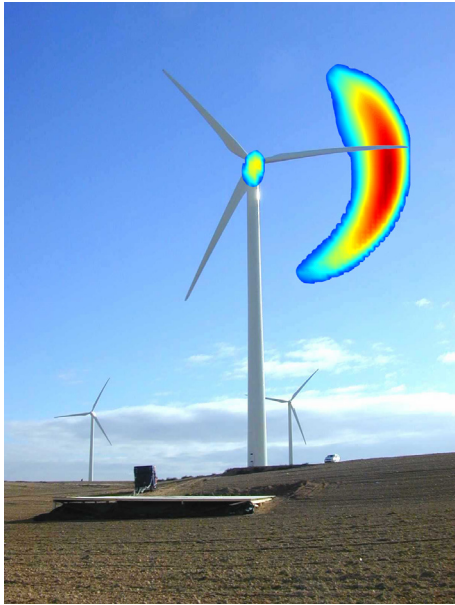
Figure 1: Picture of test set-up for acoustic measurements on the GAMESA baseline turbine. The distribution of noise sources (30 s averaged) in the rotor plane is projected onto the picture. The rotor rotates clockwise.
