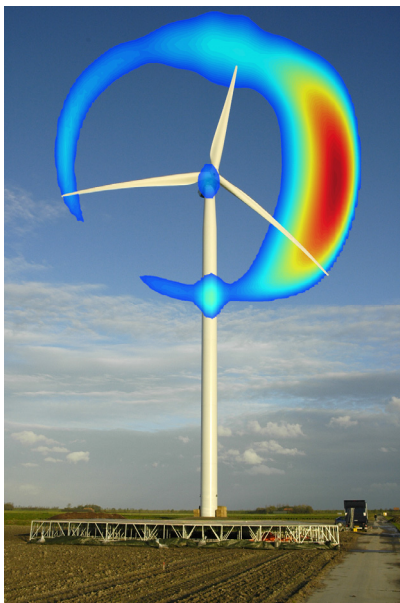
Figure 2: Picture of test set-up for acoustic measurements on the GE baseline turbine. The distribution of noise sources (30 s averaged) in the rotor plane is projected onto the picture. The rotor rotates clockwise.
