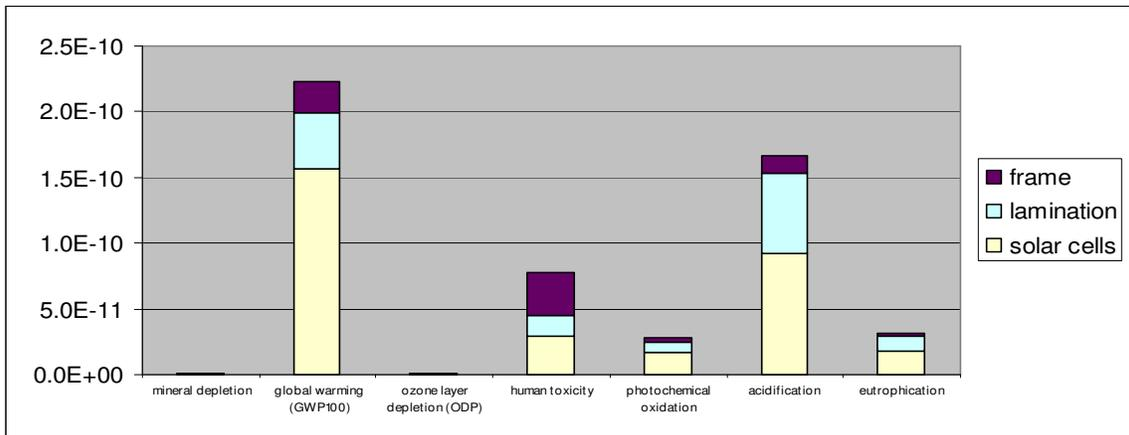
Figure 1: Normalized environmental impacts of 1 kWp of multi-crystalline silicon modules (CML 2000 method, normalisation W-Europe 1995, adapted depletion score<sup>1</sup>)
