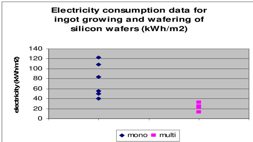
**Figure 5:** Variation in electricity consumption between different ingot/wafer manufacturers. Wafer thickness 240-270  $\mu$ m for mono-Si wafers, 200-240  $\mu$ m for multi-Si.
