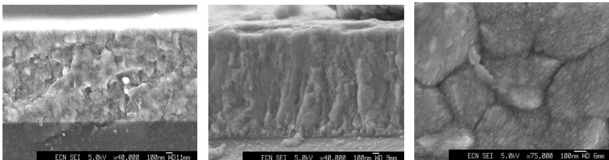
Fig. 4. From left to right: SEM cross section of ZnO:In (A) (x40.000) and cross section (x40.000) and top view (x75.000) of (i-ZnO)/ZnO:In (B)
