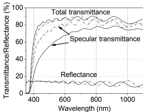
Fig. 6. UV-VIS spectra of ZnO:In (A) (solid lines) and (i-ZnO)/ZnO:In (B) (dash-dotted lines) (The layer thickness is 1300 nm).
