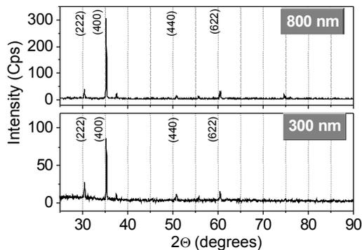
Fig.2. X-ray diffraction spectra of a 300 nm and 800 nm thick ITO layer
