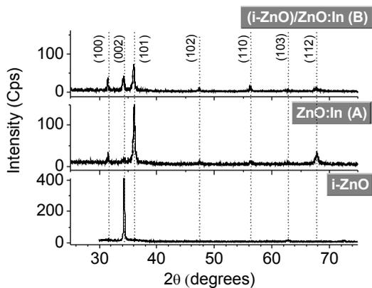
Fig. 5. X-ray diffraction spectra (coupled scan) of i-ZnO, ZnO:In (A) and (i-ZnO)/ZnO:In (B)
