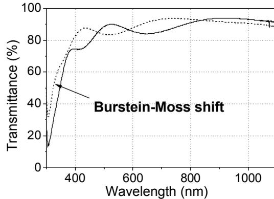
Fig.3 UV-VIS transmittance spectrum of an as-deposited (solid line) and forming gas annealed (dotted line) ITO layer (layer thickness: 300 nm)
