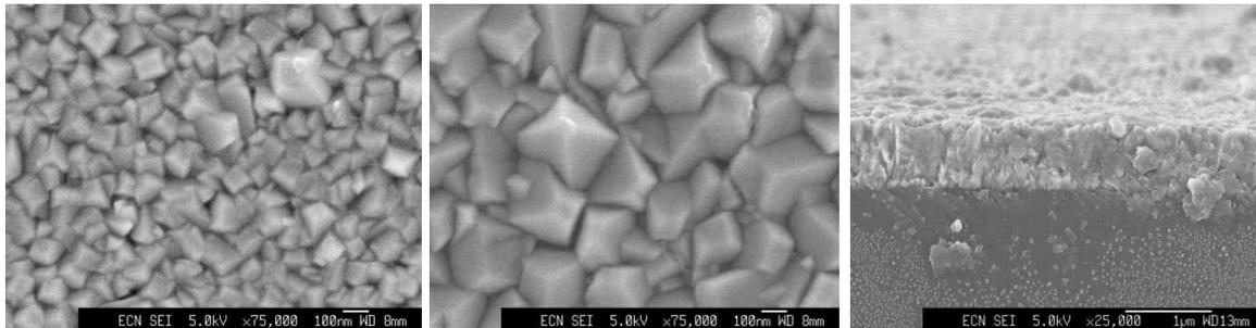
Figure 1 From left to right: SEM top view of a 300 nm thick ITO layer (x75.000) and SEM-top view (x75.000) and cross section (x50.000) of a 800 nm thick ITO layer
