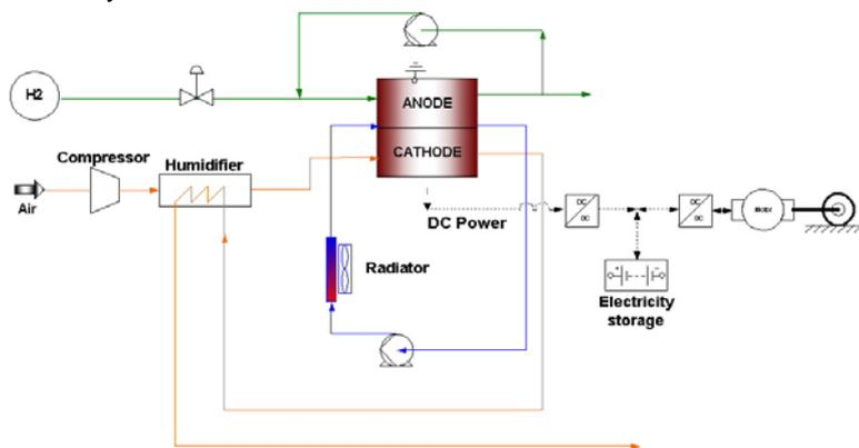
**Figure 1. Simplified Process Flow Diagram of the hybrid Fuel Cell/Electricity storage system**
