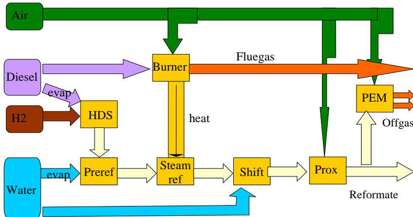
**Figure 2. Simplified block diagram 25 kW demonstrator for diesel reforming**
