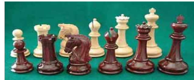
White pieces from combustion fly ash Black pieces from gasification fly ash
